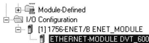
**Figure 14: DVT System added as to the I/O Tree in a ControlLogix system**
